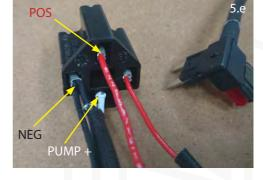
5.f. Plug in the connector onto the pump.
