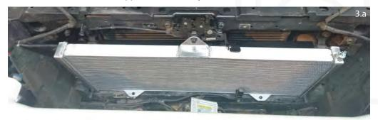
3.b. Check that the auxiliary coolers in front of the condenser do not touch the newly positioned intercooler radiator. There must be at least 10mm of clearance, if there isn't then the auxiliary cooler brackets will need to be slightly modified towards the engine.
