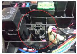
5.i. Remove the "Fuel Injector" fuse, replace the 10 Amp fuse in the "add a circuit fuse tap" harness and plug it in the injector fuse slot.
