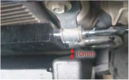
3.c. Now mark the holes that need to be drilled for the cooler hoses, these should be inline height wise with the pipes from the intercooler radiator. They will need to be over towards the right to clear the engine radiator. Drill a 30-32mm hole in the side seals. Image is of the lower hole, once lower hole is correct mark up a distance of 155mm for top hole. Note measurements are a guide only.
