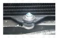
3.e. Finally double check that the core has a minimum of 10mm of clearance from accessories including the ambient temperature sensor.
